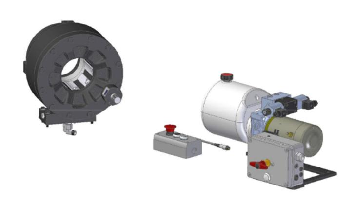
The NKS-40 is a splitted version of our NK40 hose crimper, specially designed for kitting mobile vans. The head must be linked to the hydraulic unit by 2 hose assemblies 3/8" size (3/8" BSP Ports). The kit is supplied with 2.5 metre long electric cable to link the electric box to the control box. The NKS concept allows to optimize the space and the weight in the hose repair vans. The NKS40 is available in different electric voltages 12V, 24V, 110V, 220V 1-PH or 400V 3-PH
